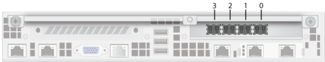
Figure 6. Quad 10 GbE SFP+ input/output connectors (option)
