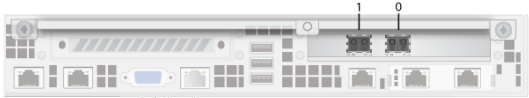
Figure 5. Dual 25 GbE SFP+ input connectors (option)
