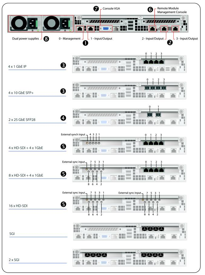
Note that the back panel components are SELV (Safety Extra Low Voltage) components.
